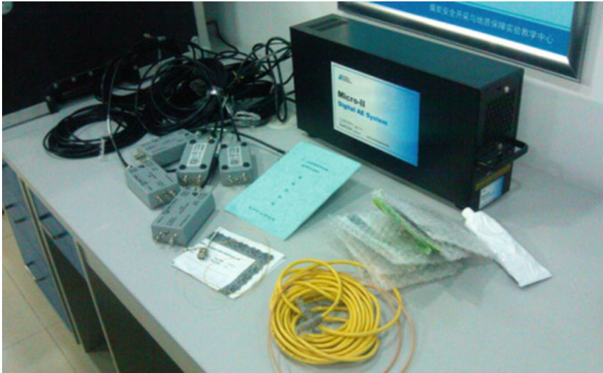
Fig. 2.4 PCI-II AE testing system
