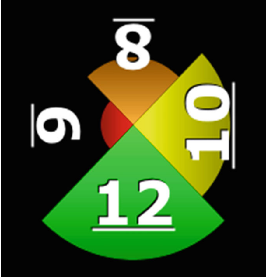
Fig. 12.2 The graphical performance feedback in the center of the interface, showing in real time the number of ideas produced by each group member around the table
