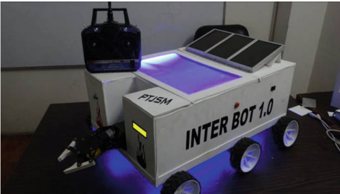
Fig. 14. InterBot 1.0 robot with 2.4 GHz 6-channel transmitter
