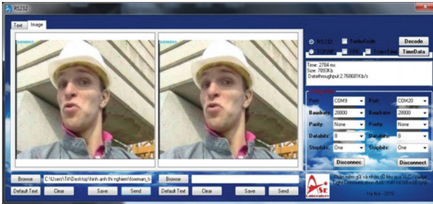
Fig. 6. GUI experimental software: image-information transmission mode at distance of 2.4 m, file size of 17.133 kb, and baudrate of 28.8 kbps
