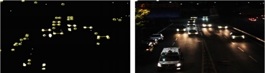
Fig. 13. A result of car headlight detection and pairing
