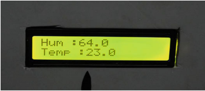
Fig. 7. Temperature and humidity display on LCD
