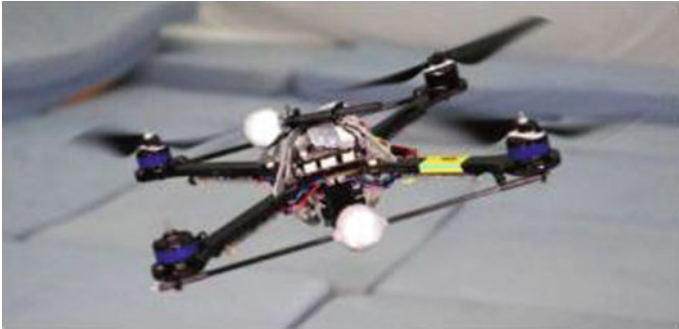
Fig. 1. Quad copter in controlled flight despite losing one rotor. Stability augmentation system is based on this model
