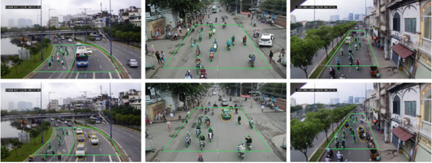
Fig. 5. Examples of occlusion vehicle detection and classification result with three experimental datasets. Green, yellow, blue ellipses, respectively, indicate light, medium, and heavy vehicles. On the 1st column: results from dataset HMD01. On the 2nd column: results from dataset NTL01. On the 3rd column: results from dataset COL01
