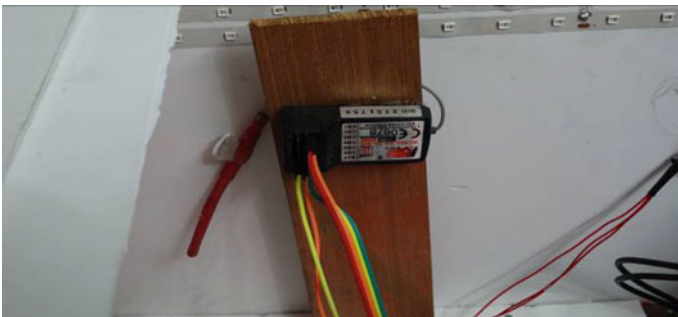
Fig. 12. 2.4 GHz 6-channel receiver
