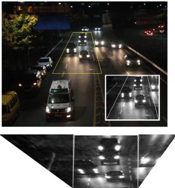
Fig. 7. A nighttime traffic scene with a perspective transformed region
