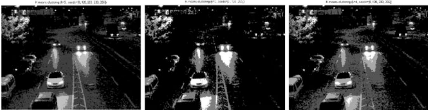
Fig. 6. Brightness layers from k-means clustering with k = 3, 4, 5 (from left to right, respectively)
