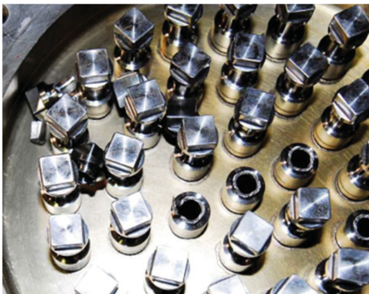
Fig. 16 Damaged rocket motor injector shear [48]
