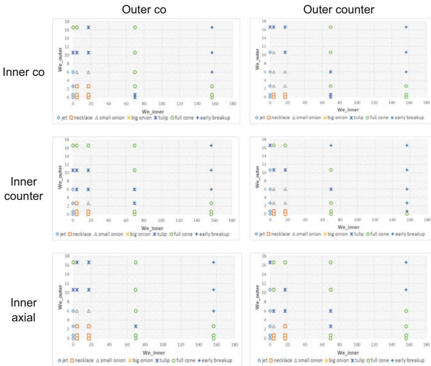
Fig. 9.9 Breakup regimes for developing spray on 1 LPM 10% ethanol-blended kerosene flow
