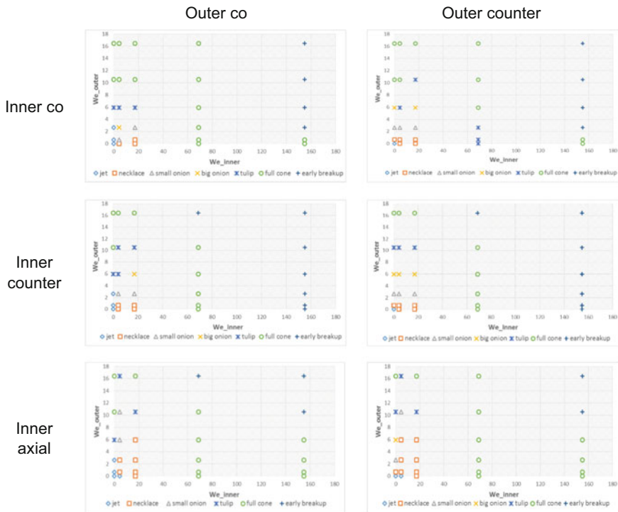
Fig. 9.5 Breakup regimes for developing spray on 1 LPM kerosene flow
