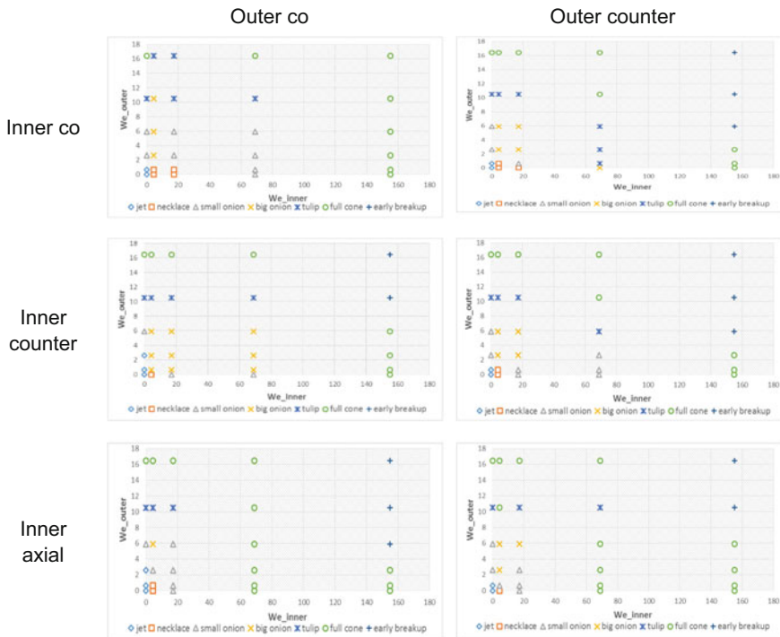
Fig. 9.6 Breakup regimes for developing spray on 2 LPM kerosene flow
