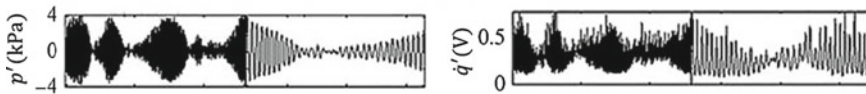
Fig. 14.3 The variation of acoustic pressure and heat release rate fluctuations obtained during a state of intermittency observed prior to a flame blowout in a bluff-body-stabilized turbulent combustor. The flow conditions were Re = 2.28 \times 10^4 and equivalence ratio = 0.47. During intermittency, both acoustic pressure and heat release rate fluctuations show apparently random switching between bursts of high amplitude periodic oscillations amongst the regions of low amplitude aperiodic oscillations (Unni and Sujith 2015)
