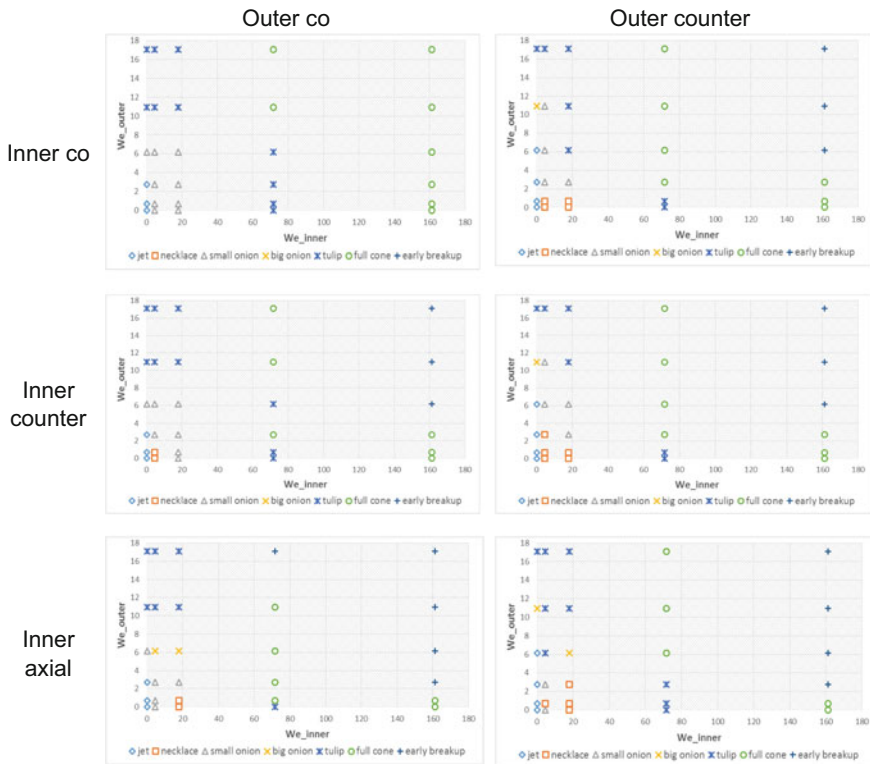
Fig. 9.8 Breakup regimes for developing spray on 2 LPM ethanol flow
