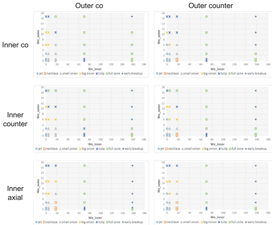
Fig. 9.12 Breakup regimes for developing spray on 2 LPM 20% ethanol-blended kerosene flow
