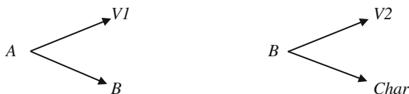
Fig. 3 Decomposition of hemicelluloses; A—xylan (major component in hemicellulose), B—intermediate reaction product with a reduced degree of polymerization and V1, V2—volatiles produced during reactions (Di Blasi and Lanzetta 1997)
