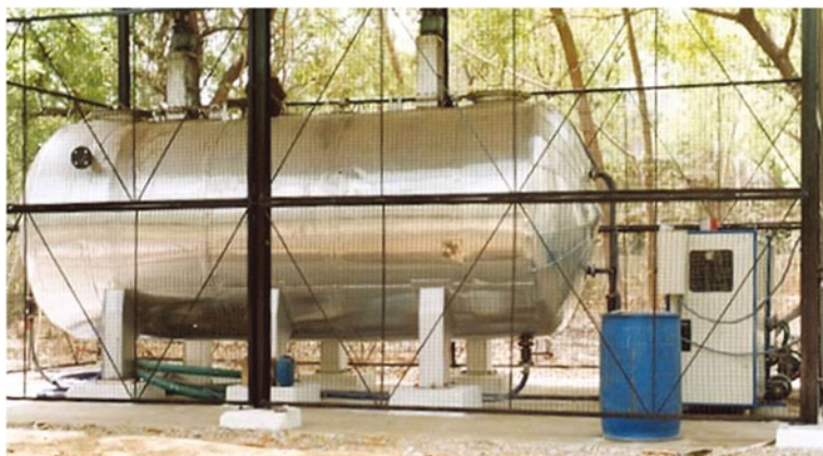
Fig. 2 Anaerobic microbial inoculum generation facility (14 m 3 capacity) in operation at Defence R&D establishment, Gwalior, India. Source Singh and Kamboj (2018)
