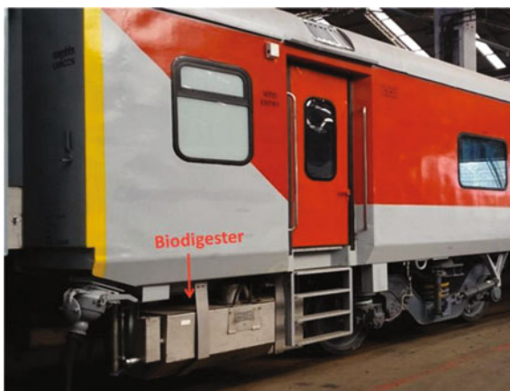
Fig. 4 Biodigester fitted under an Indian train coach
