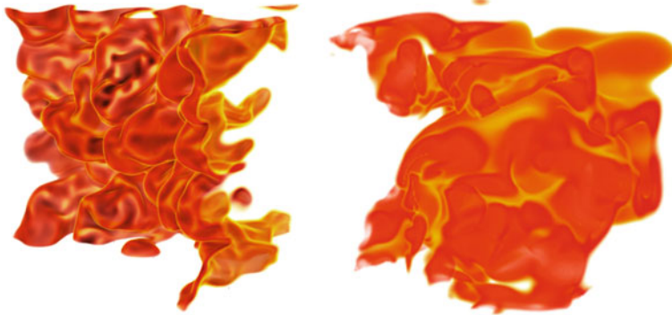
Fig. 4.7 Instantaneous images of the heat release rate isocontours for statistically stationary turbulent premixed hydrogen–air flames at Ka = 14 (left) and 126 (right), representing the corrugated laminar flamelet and distributed combustion regimes, respectively (Im et al. 2016)
