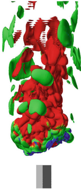
Fig. 4.11 Global structure of the hydrogen jet lifted flame. Surface color shows the combustion mode: red (rich premixed), blue (lean premixed), and green (nonpremixed) (Mizobuchi 2005)
