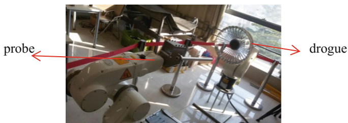
Fig. 3. Data acquisition system. It is consisted of two robots, one plays the role of flying tanker, we installed a drogue on its flange, the other one plays the role of receiver aircraft, we installed a camera on its flange. Pose information of drogue can be read from controller, we use this as ground-truth to validate our pose measurement framework.
