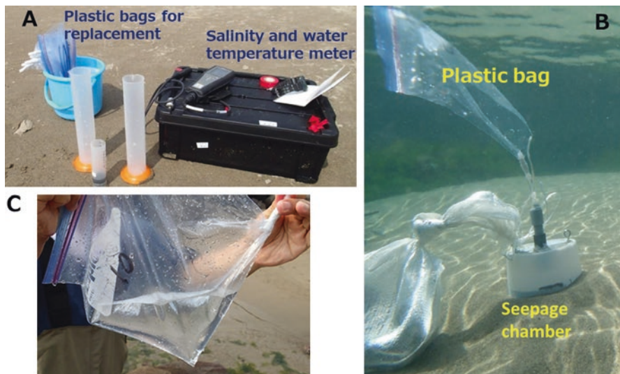
Fig. 9.4 Photographs of seepage meter used in study areas (A) tools to measure the SGD flow rate and freshwater ratio in SGD, (B) seepage meter installed in the field, and (C) seepage water stored in the plastic bag
