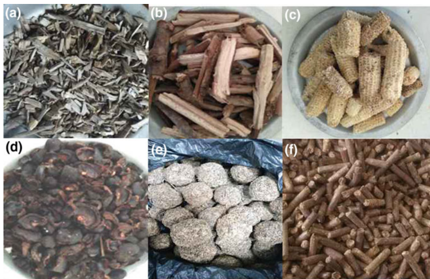
Fig. 3 Fuels that can be used in HC3D combustion systems: a cut tree droppings along with bark, packing density of 200 to 210 kg/m 3 , b casuarina chopped pieces, packing density of 240 to 280 kg/m 3 , c corncobs, packing density of 200 to 210 kg/m 3 , d cashew shell waste—90 to 100 kg/m 3 , e processed sawdust—cowdung balls, 60 to 80 kg/m 3 , f pellets of a mix of seasonal agro-residues, packing density = 600 kg/m 3 , ash content of all biomass ≤ 5%
