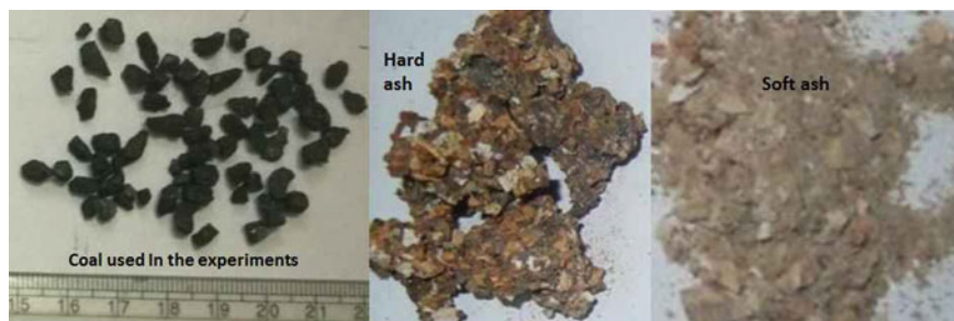
Fig. 10 Coal pieces, hard ash (with some unconverted carbon), and soft ash found in the experiments
