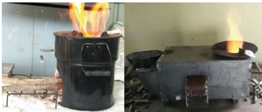
Fig. 7 Comparison between the flames behavior of a free convection stove and the single-pan forced convection single-pan stove (HC3D design)
