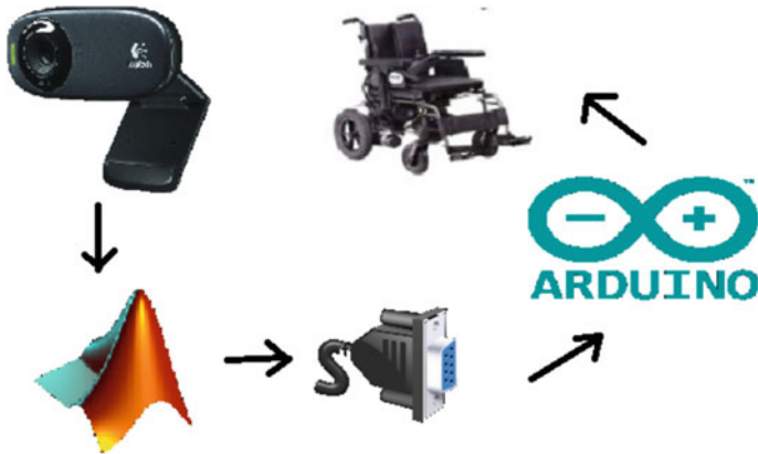
Fig. 1 Basic architecture of automated eye-tracking system
