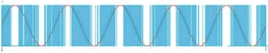
Fig. 7 Digitized sine wave by Zoom ADC converter
