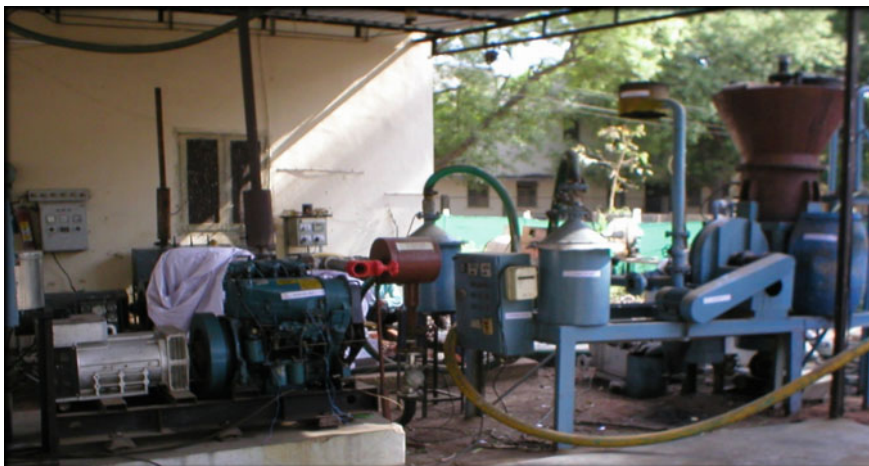
Fig. 13 Gasifier based CI engine for dual-fuel operation (Singh 2007)
