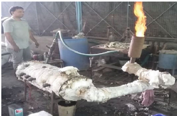
Fig. 10 Horizontal gasifier (Singh et al. 2016)
