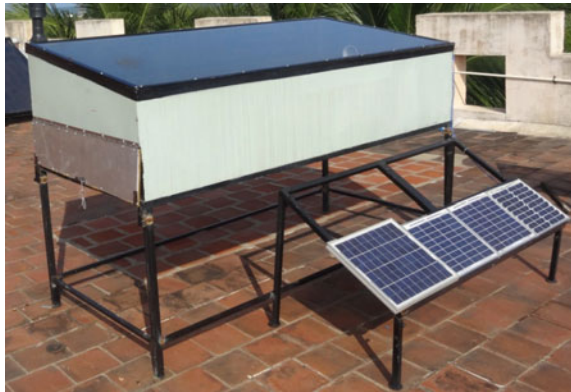
Fig. 9 Solar tunnel dryer (Rajarajeswari et al. 2016)
