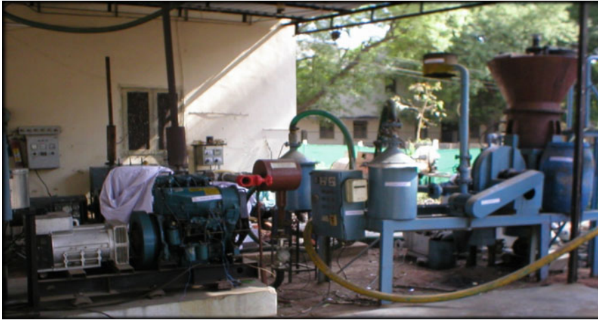
Fig. 13 Gasifier based CI engine for dual-fuel operation (Singh 2007)
