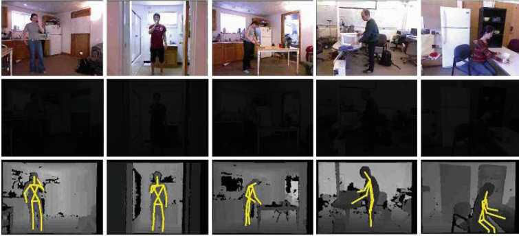
Fig. 1. Illustration of RGB and depth images. Row 1 shows the RGB images in the bright environment. Row 2 shows the RGB images in the dark environment. Row 3 shows the depth images in the dark environment.
