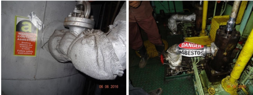
Fig. 3 Labelling of asbestos-containing material found in ship recycling industries. Before dismantling the ship, proper identification and labelling of asbestos-containing areas are done and disposal activity is further done by the licensed asbestos contractors
