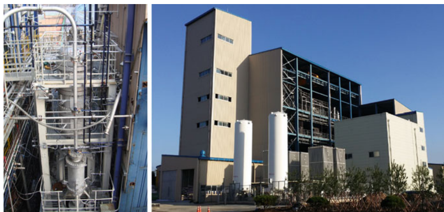
Fig. 2 Coal gasification pilot (left, 3 ton/day) and demo test-bed (right, 20 ton/day) plants at Institute for Advanced Engineering in Korea
