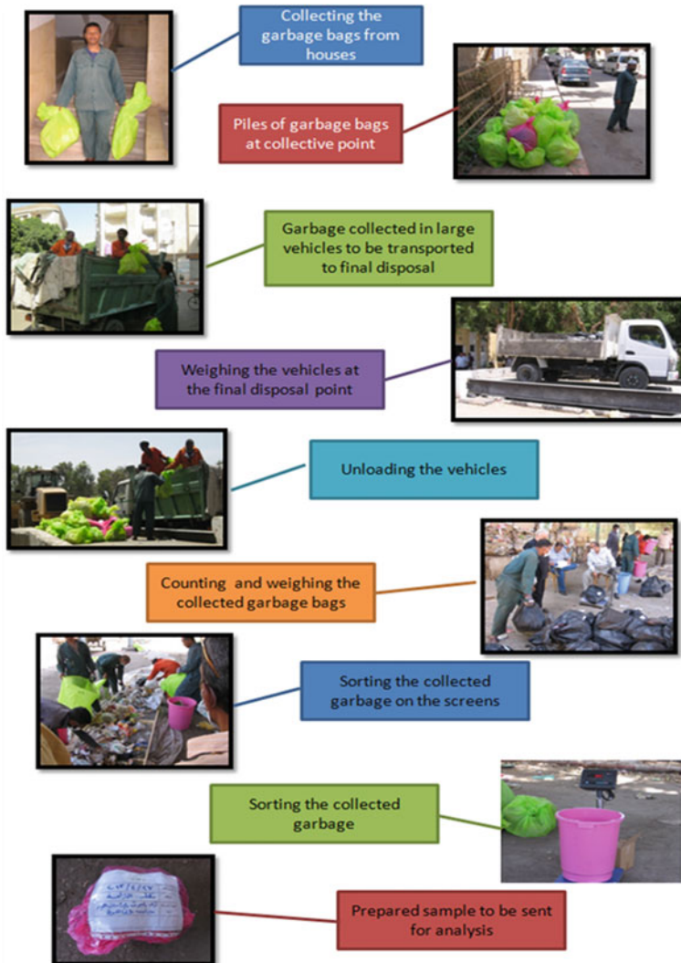
Fig. 1 A schematic diagram showing the steps followed in MSW collection and characterization
