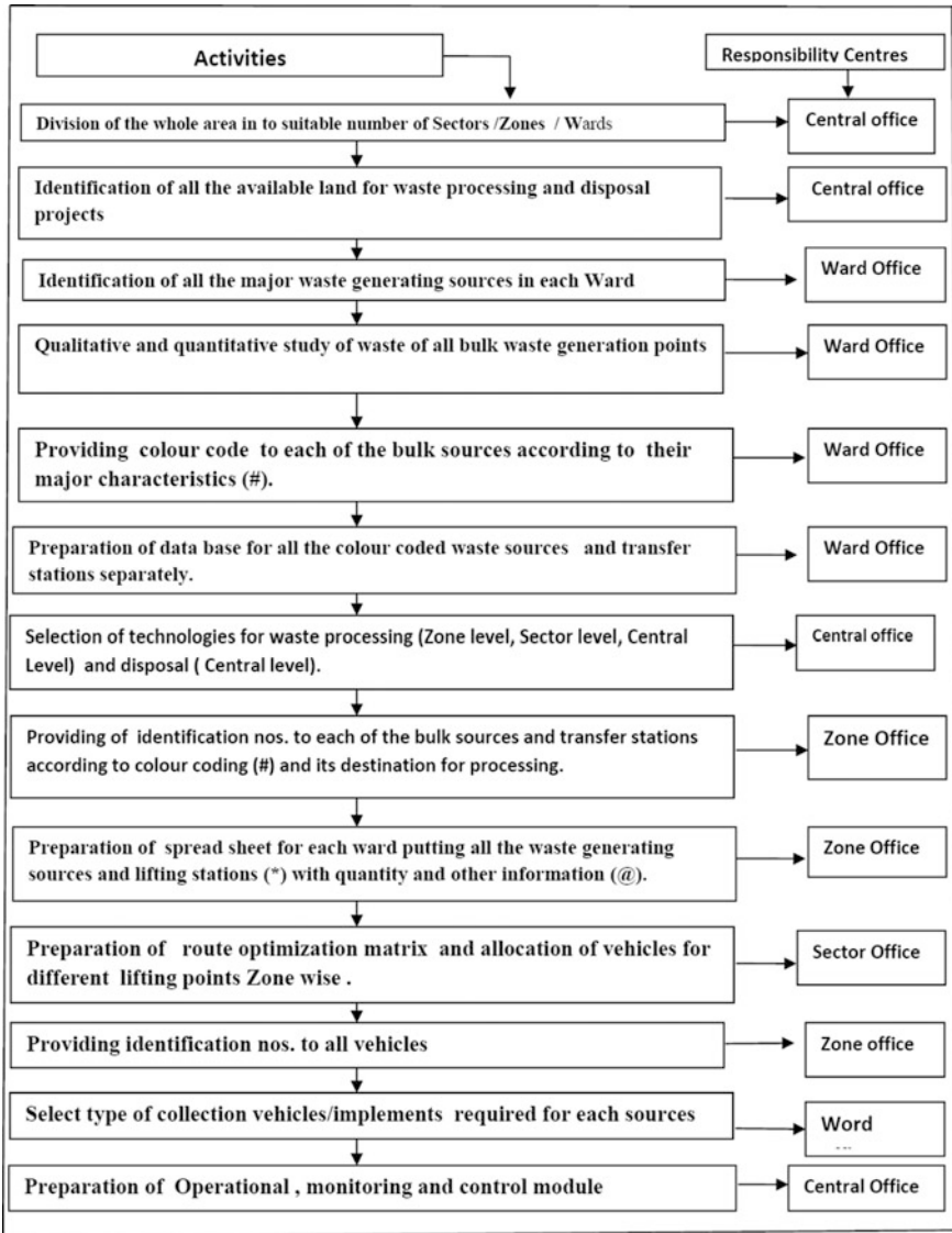
Fig. 4 Flowchart for activities of responsibilities for planning and development of MSWPD system. (@) Information such as location, color code, approximate quantity of daily waste, distance from the disposal ground, vehicle type, vehicle’s garage. (*) Also locate all the major sources in ward maps as per their color code. (#) Color code as prescribed above
