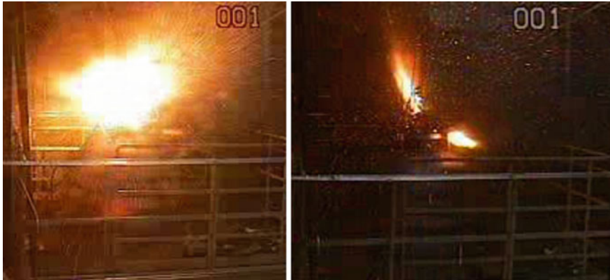
Fig. 6 Explosion moments at the coal feeding nozzle area during the pilot gasifier operation at IAE (20 bar, 1,400 °C). Left: explosion at the nozzle area, (right) remaining explosion gas leaks out after a short explosion as in the left picture
