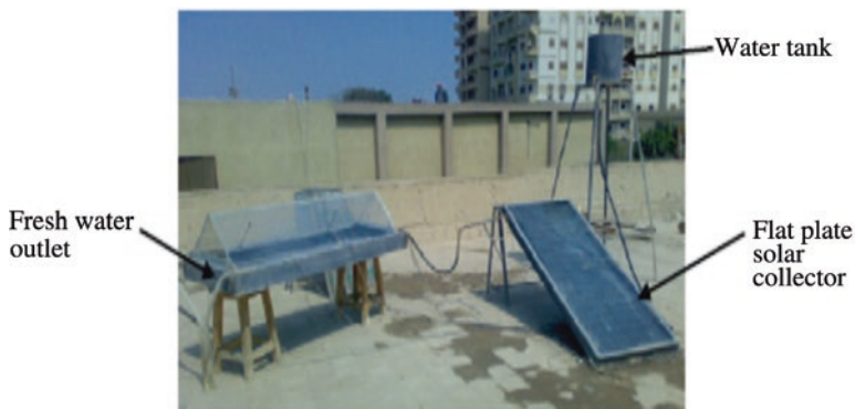
Fig. 14.11 Active solar still coupled with flat plate collector (FPC) (Morad et al. 2015)
