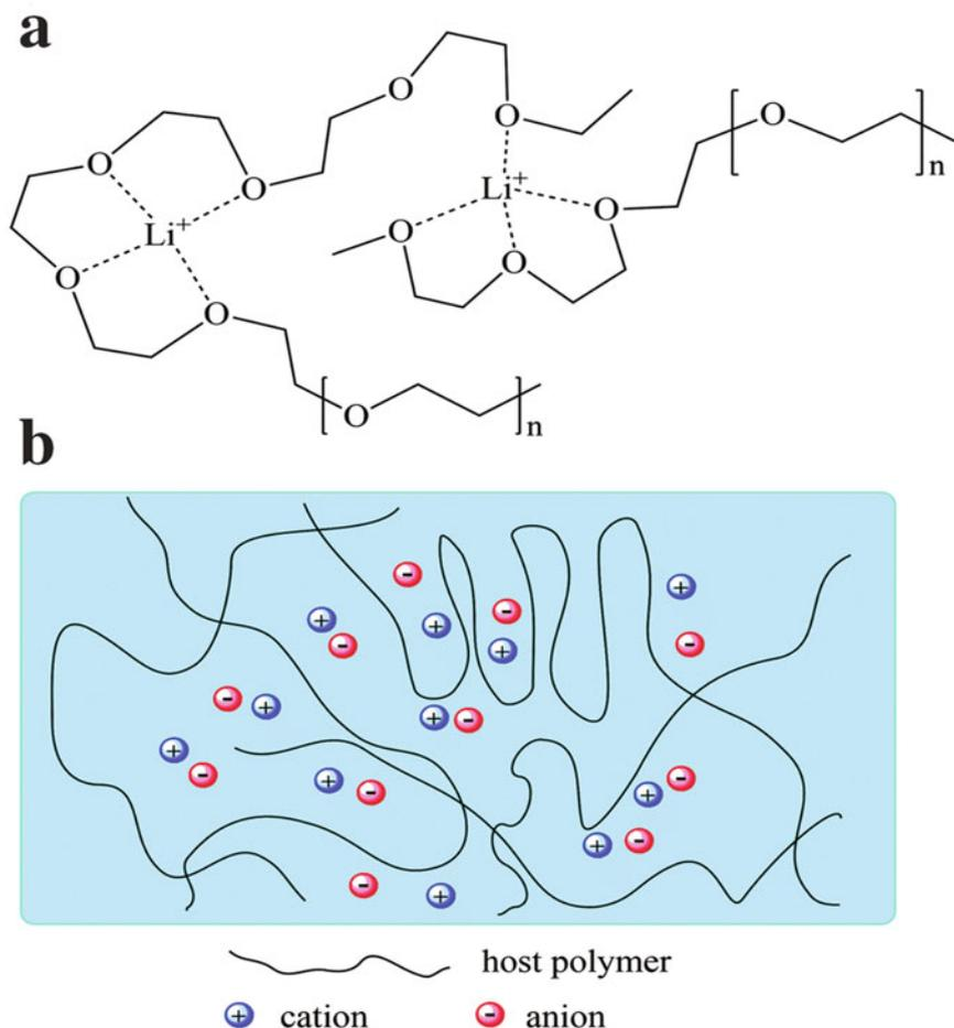
**Fig. 3.6** Schematic showing **a** a solid polymer electrolyte and **b** gel polymer electrolyte. Reproduced with permission from Zhong et al. (2015a)
