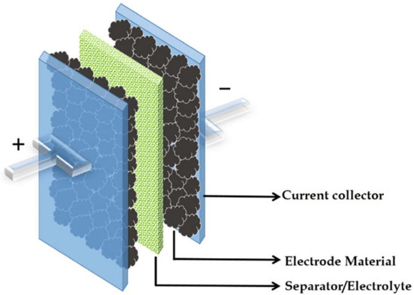
Fig. 3.1 Components of supercapacitor
