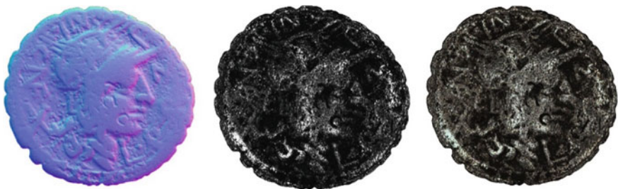
Fig. 14 Specular components for coin obverse: (left) normals; (centre) quotient; (right) colour
