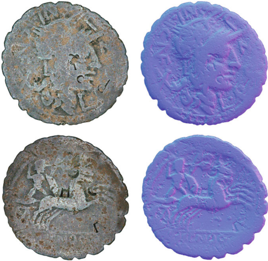
Fig. 12 Albedo and normals of the coin, derived from processing the sets of 64 images
