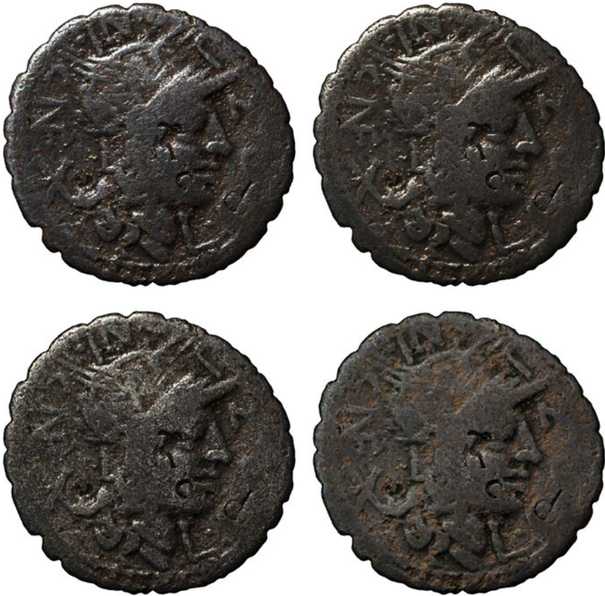
Fig. 24 Rendering of coin images illuminated by a single lamp: (top left) photographic image; (top right) power Lorentzian model; (bottom left) previous cluster Lorentzian model; (bottom right) Lambertian model
