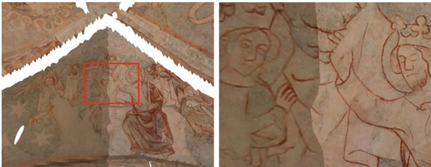
Fig. 5 A wide and short telephoto image used for texturing the mesh, viewed in a split way. The added detail of the tele image is clearly visible. White regions were not visible from any camera's point of view, therefore are not colorized
