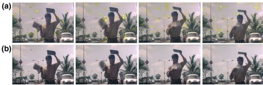
Fig. 10 a Naturally degraded frames with PCA and blotches; b respective restored frames after restoration of PCA and blotches
