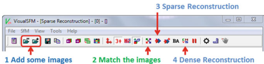
Fig. 1 Different steps of the pipeline of a 3D reconstruction process using the VisualSFM
