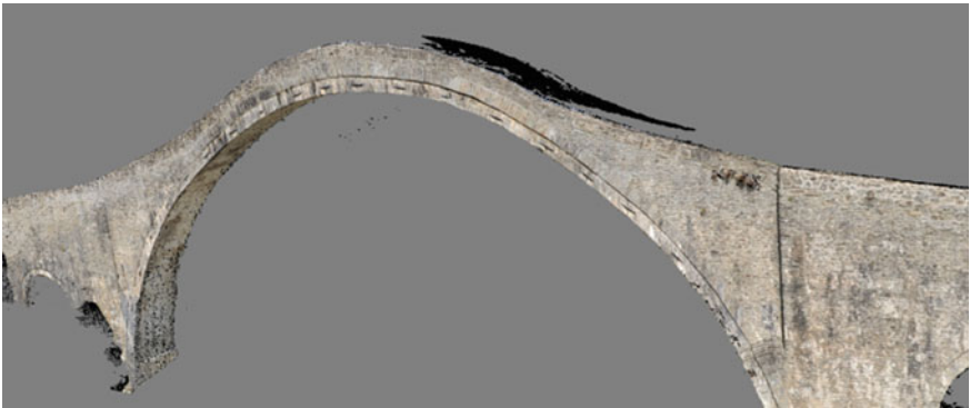
Fig. 10 A view of the textured mesh created in Agisoft PhotoScan
