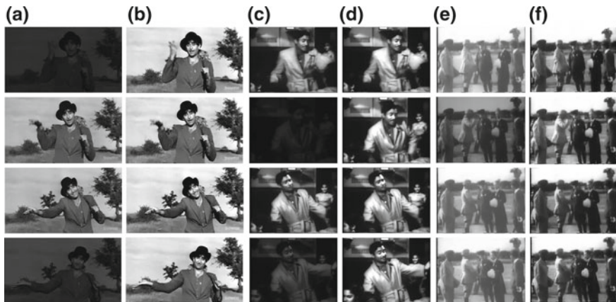
Fig. 7 a , c and e frames from videos having intensity flicker; b , d , and f frames of the respective videos after restoration
