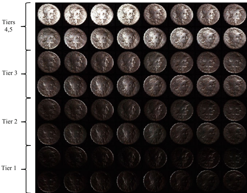
Fig. 9 Montage of 64 images of the obverse of the Roman denarius, taken by a Nikon D200 camera in the UCL dome, illuminated by each of the 64 flashlights arranged in five tiers. The image brightness decreases with angle of elevation of the light source, shown from top of the figure (highest angles in Tiers 4, 5) to the bottom (lowest angles in Tier 1)
