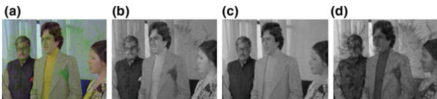
Fig. 4 Partial color artifacts: a RGB frame; b R plane; c G plane; d B plane
