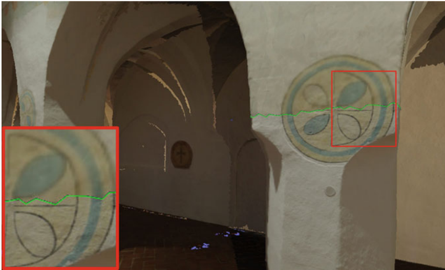
Fig. 6 Model textured with distant images, while a close-up image brings significant improvement in resolution, as seen on the bottom part of the pillar. Green line marks the texture boundary
