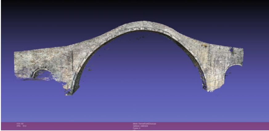
Fig. 9 Dense point cloud produced in Agisoft PhotoScan—56 images
