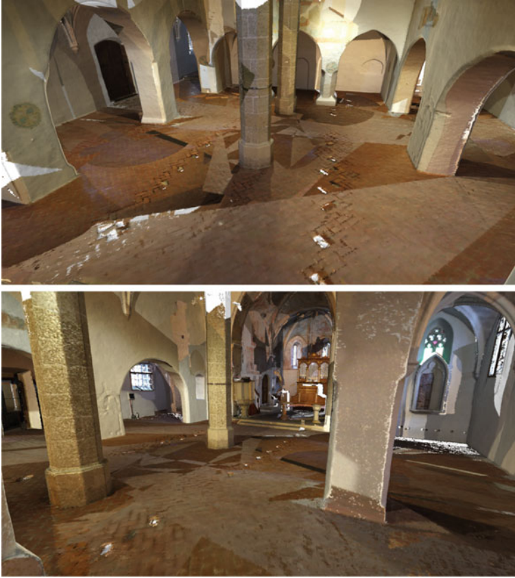
Fig. 7 Overview of the colorized interior using the vertex-based method. Some white balance and exposure correction has been done on the camera images
