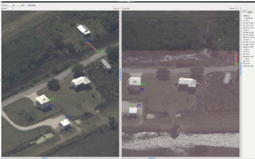
Fig. 9 Multi-pair measurement interface: 3 measurements in a pottery dataset, and b Louisiana dataset. Each measurement is marked in red line segment together with two endpoints, one in green and one in blue. Each pair of points in two images with the same label are matched feature points. Distance for each line segment is displayed on the right side
