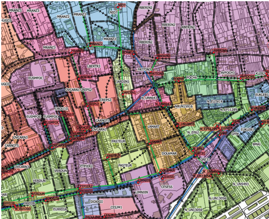
Fig. 2 Extract from a map of design drainage areas in a 1D model, showing the pipe route and the injection points on the network (urban hydrological modeling)
