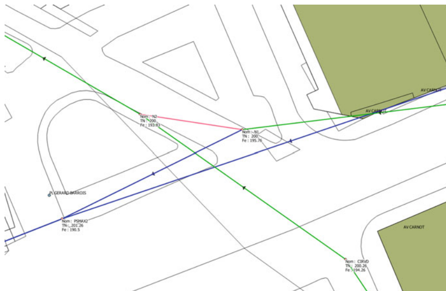
Fig. 3 Extract from a map in a 1D model, showing propagation in the network. In this case, a stormwater regulator
