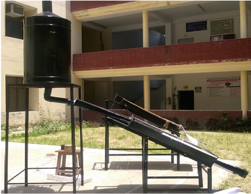
Fig. 6 A solar chimney fruit dryer with a solar air heater (consisting of single or double glazing, a solar collector, an air blower, ducts for air supply, and sometime a PV module in case of hybrid solar dryer)
