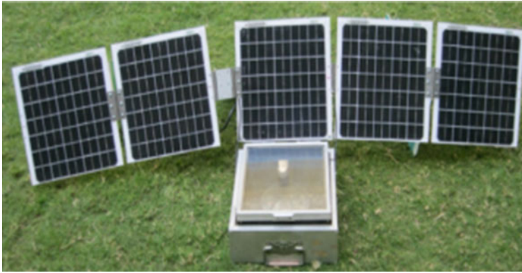
Fig. 11 Experimental setup of a hybrid solar cooker [103]
