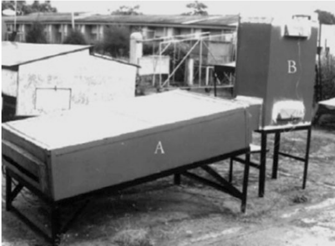
Fig. 15 Photograph of the air-heating system. A, Collector assembly with energy storage and air-heating subsystems; B, heated space [29]
