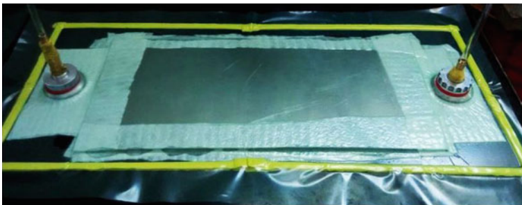
Fig. 5 Casting of composite panel using vacuum bagging technique
