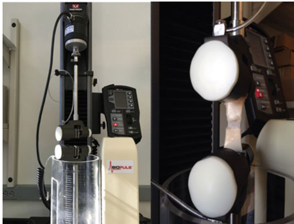
Fig. 1 Instron testing system equipped with a Bioplus bath and a picture of a tested specimen
