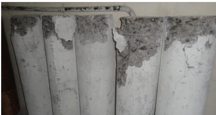
Fig. 5 Failure pattern of unwrapped column specimen
