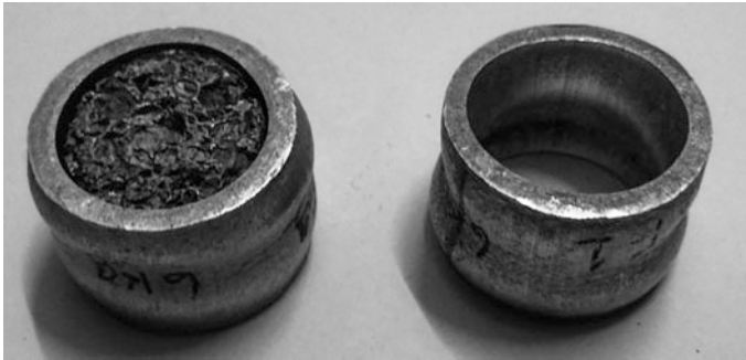
Fig. 11 Deformed shape of empty and aluminum foam-filled AA7075-T6 tubes after dynamic compression
