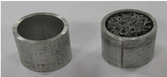
Fig. 2 Empty and aluminum foam-filled AA7075-T6 tubes
