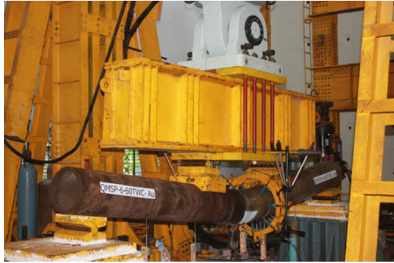
Fig. 6 Deflected shape of the specimen QMSP-6-60TWC-Au at the end of fracture test
