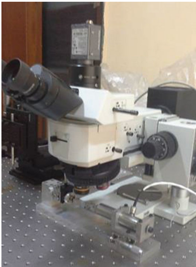
Fig. 3 In situ optical micro-tensile setup
