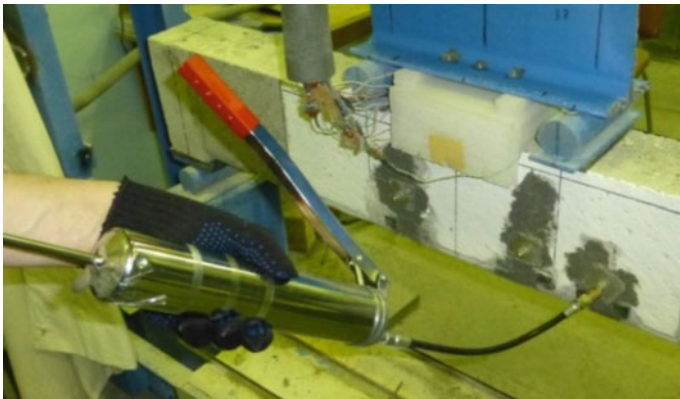
Fig. 2 Epoxy crack injection
