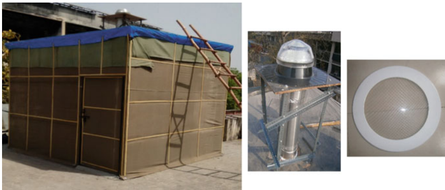
(a) Test room with light pipe set-up (b) Light pipe with dome (c) Diffuser
