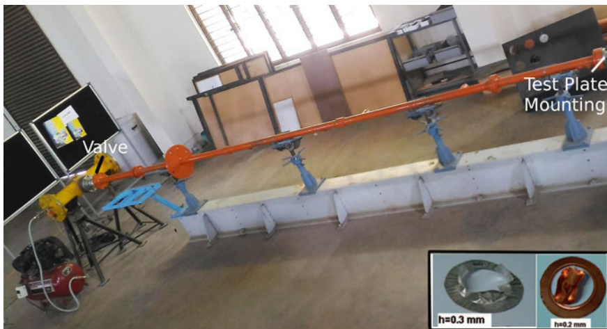
Fig. 10 A photograph of the diaphragmless shock tube at IISc. The inset at the lower right shows failed aluminum and copper samples. The loading area was \phi 50 mm
