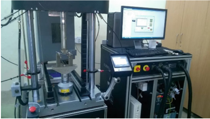
Fig. 5 Three-point bend flexural test setup
