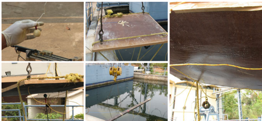
Fig. 1 Experiments carried out at National Underwater explosive testing facility at Naval Science and technology Limited, Defence Labs, Vishakhapatnam, India. The figures show the PETN explosive charge, arrangement of attachment to the sandwich composite panel, attachments of pressure transducers above the panel, immersion of the system underwater. The dimpled shape demonstrates the deformations sustained by the sandwich composite panel subjected to an real underwater explosion
