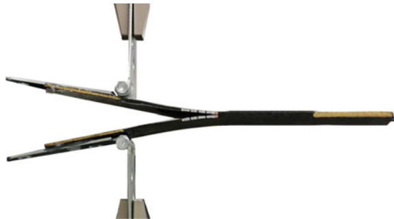
Fig. 3 DCB test in progress of a carbon fiber laminate with ZnO nanowires
