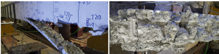
Fig. 4 Cover delamination at the constant moment region of strengthened beams
