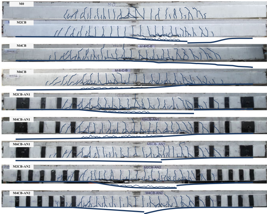
Fig. 5 Crack patterns of test beams
