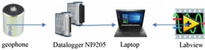
Fig. 7 Block diagram for vibration measurement system
