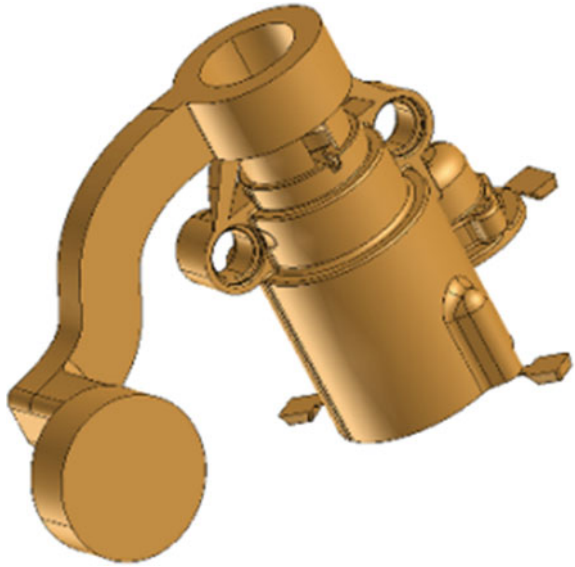
Fig. 7 Die casting with full inlet
