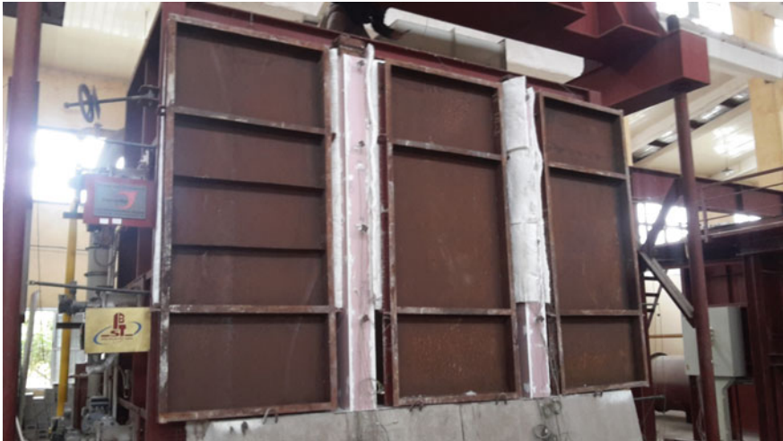
Fig. 8 02 steel column protected by gypsum plasterboard 12.7 and 15.8 mm (2)
