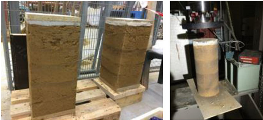
Fig. 5 Left: prismatic specimens. Right: cylindrical specimen
