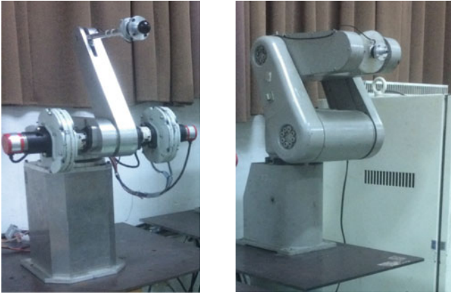
a) Manufactured haptic master b) Manufactured slave manipulator
