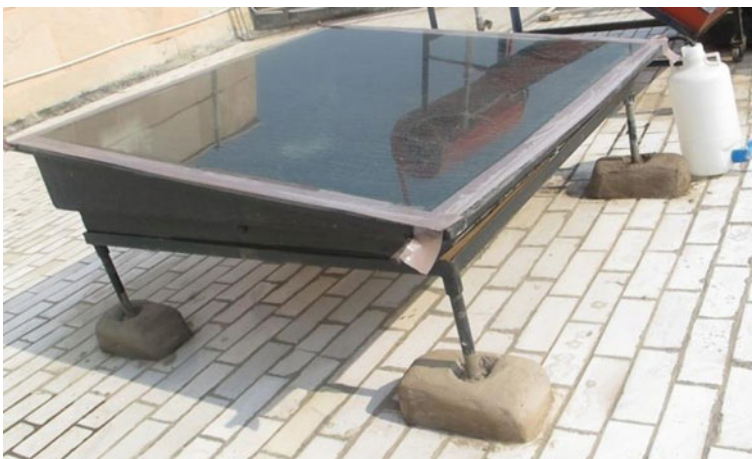
Fig. 3 Single basin-type solar still with distillate collector
