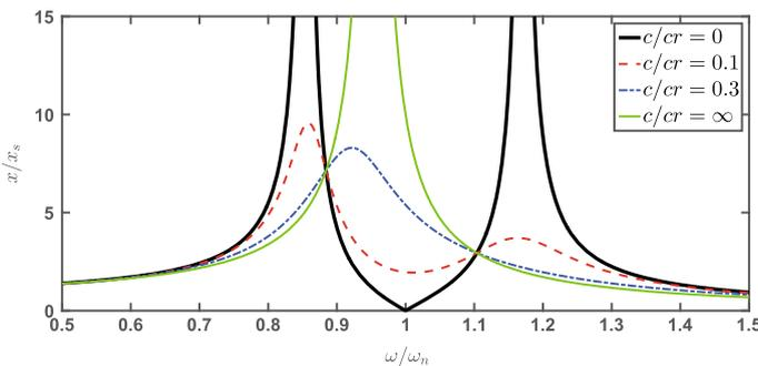
**Fig. 4.1** Frequency response of the primary mass with respect to various values of absorber damping for traditional spring–damper DVA (Den Hartog 1985)
