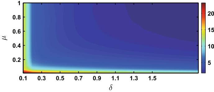
Fig. 4.7  $\max(|H_2(j\lambda)|)$  with different  $\mu$  and  $\delta$
