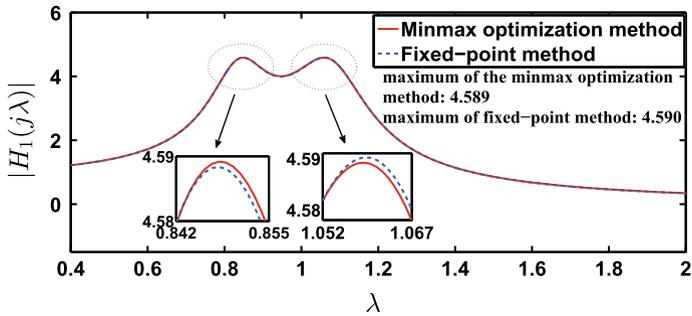
**Fig. 4.5** Comparison between the minmax optimization method in this chapter and the fixed-point method when  $\mu = 0.1$
