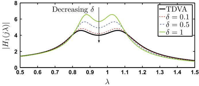
**Fig. 4.4** Comparison between the TDVA and C1 when  $\mu = 0.1$  with different  $\delta$
