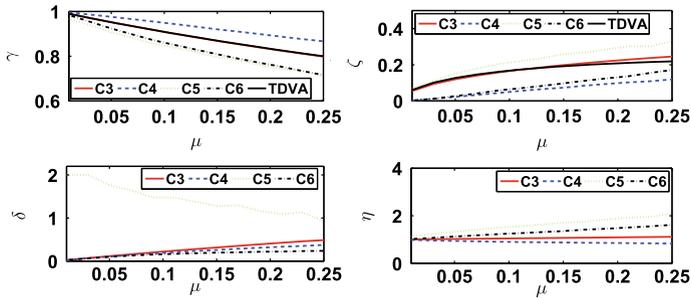
**Fig. 4.9** Optimal parameters in the  $H_\infty$  optimization: natural frequency ratio  $\gamma$  (up left); damping ratio  $\zeta$  (up right); inertance-to-mass ratio  $\delta$  (bottom left); corner frequency ratio  $\eta$  (bottom right)
