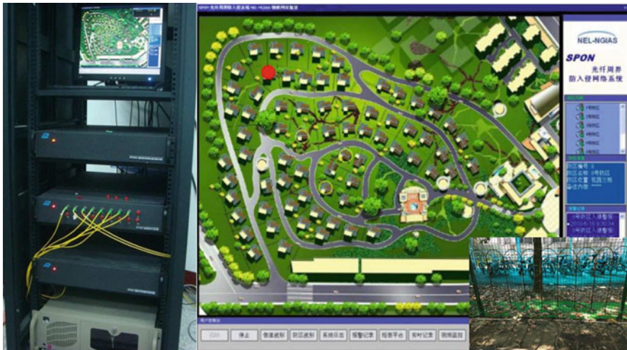
Fig. 38 Photographs of the HSPON-OLT (left) and the application software of the perimeter intrusion monitoring system (right). Inset: photo of the field test with fiber cables deployed on the ground and fence. Copyright 2019 OSA
