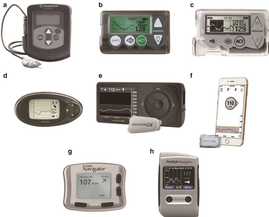
Fig. 2.1 The main CGM systems on the market. Notes: (a) Medtronic Inc. CGMS Gold; (b) Medtronic Inc. Guardian REAL-Time; (c) Medtronic Inc. Paradigm REAL-Time;
