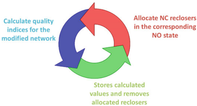
Fig. 13.4 Detail of the process of assessing the NC-AR allocation impact on the quality indices
