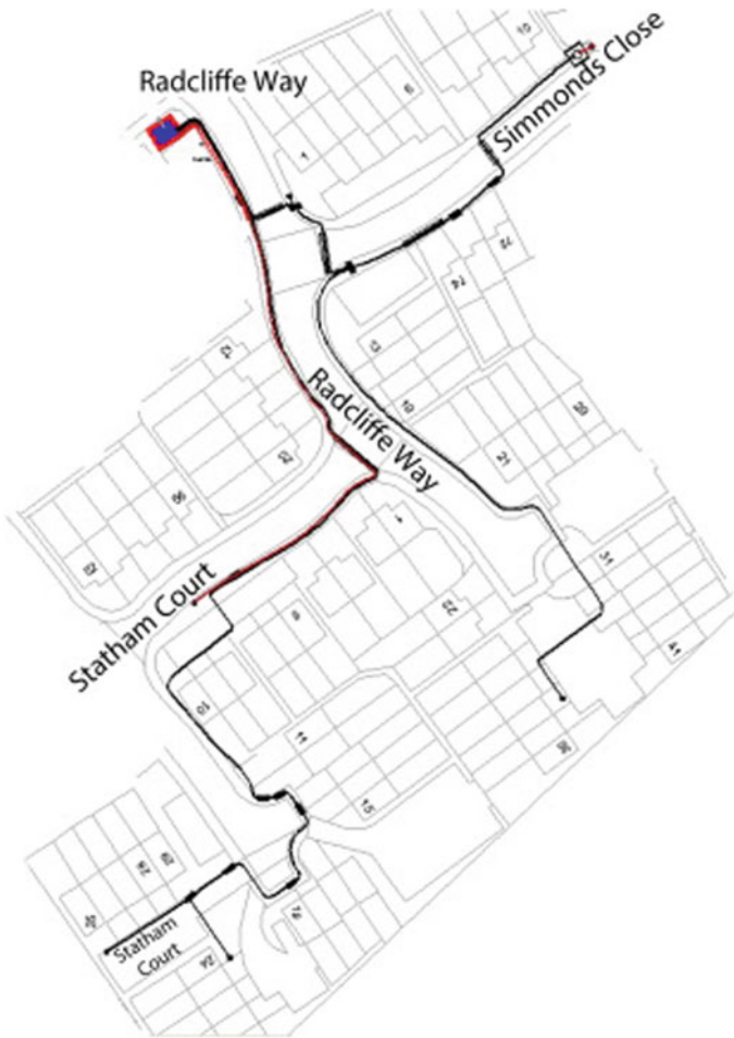
Fig. 3.2 Radcliffe way low voltage substation, Basingstoke, UK. The substation (blue) feeds residential households using three phase feeders (solid black lines) [13]
