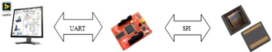
Fig. 12 Complete system using UART-SPI interface
