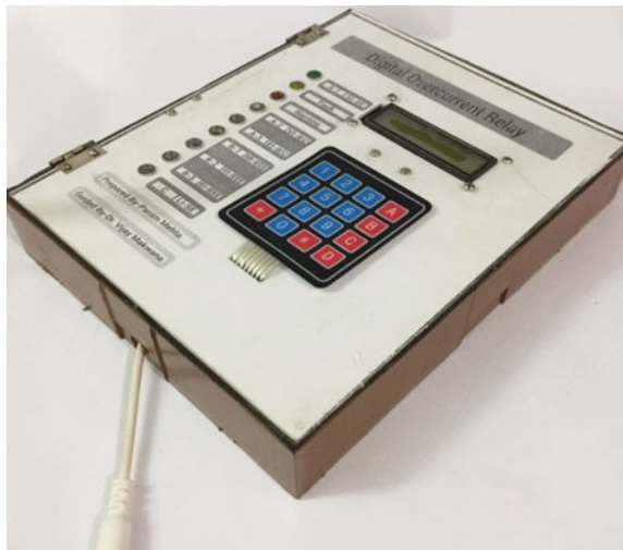
Fig. 13 Hardware model of IDMT overcurrent relay
