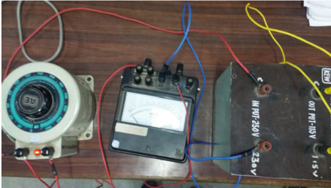
Fig. 7 Setup for short-circuit test
