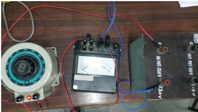
Fig. 6 Setup of open-circuit test
