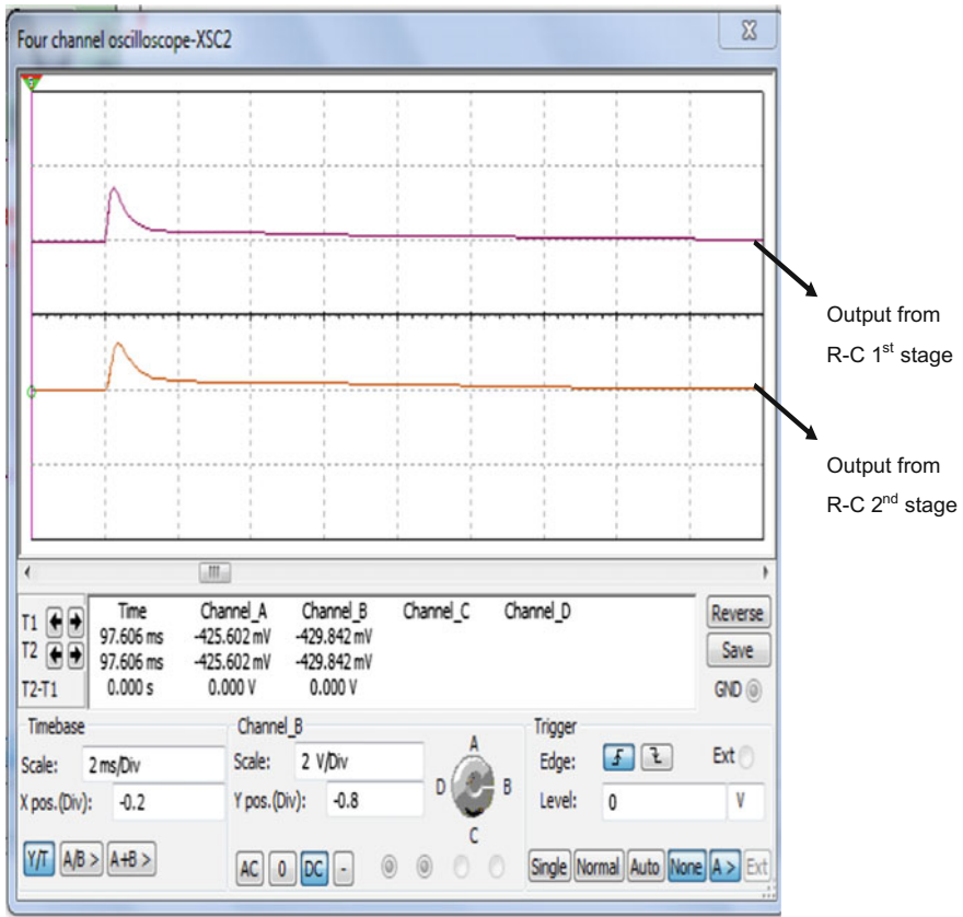
Fig. 5 Output of first and second RC stages
