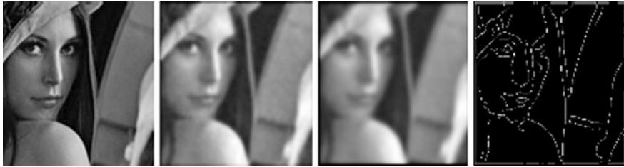
Fig. 1 Perona-Malik diffusion with static scale k = 70 a original image, b after 60 iterations, c after 120 iterations. d Canny edge of (c)
