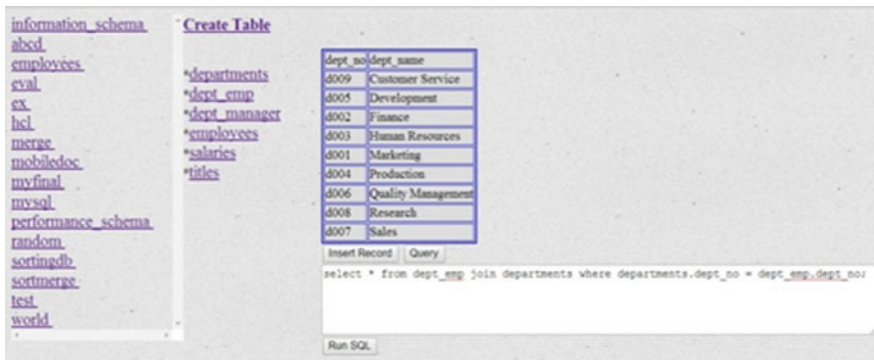
Fig. 8 Query button will allow user to type Join query only. Run SQL button will execute query
