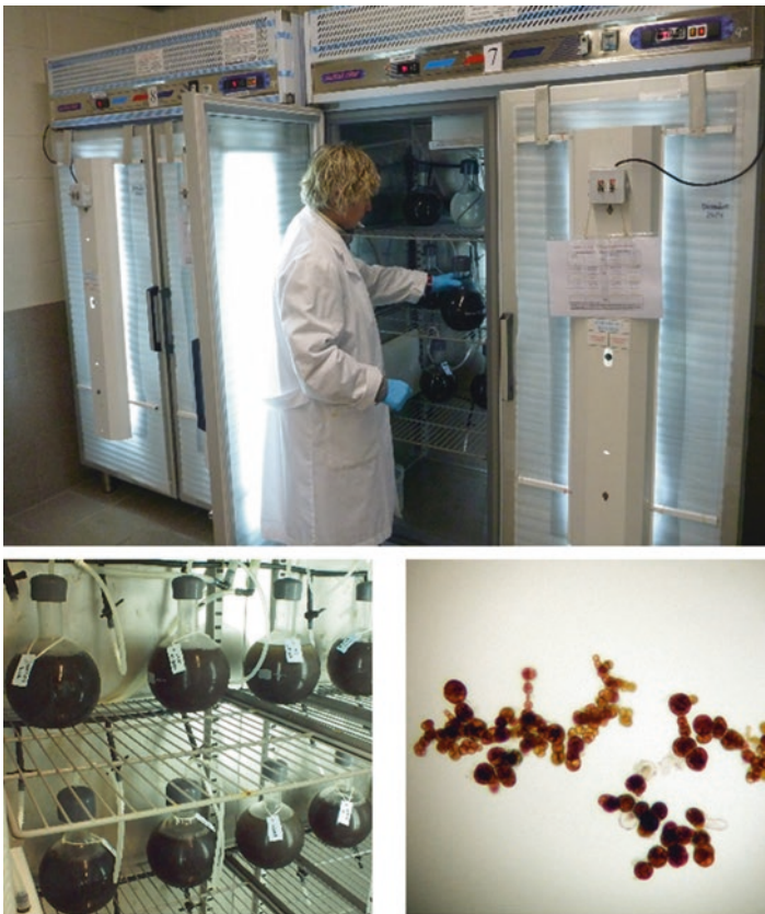
Fig. 2.13 The environmental culture chambers or incubators (above) used to maintain culture flasks (bottom left) containing microscopic kelp gametophytes (bottom right), growing under free-living conditions (Photos by C. Peteiro)
