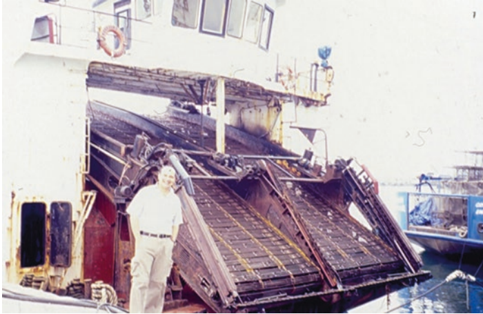
Fig. 2.9 Vessel for harvesting the kelp Macrocystis pyrifera for alginate production along the coast of California (Photo by C. Peteiro)
