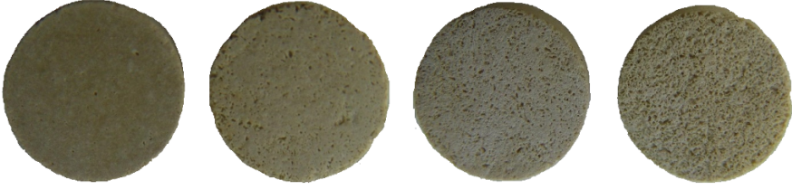
Fig. 5.2: Piezoceramics with different size of pores and pores percentage.
