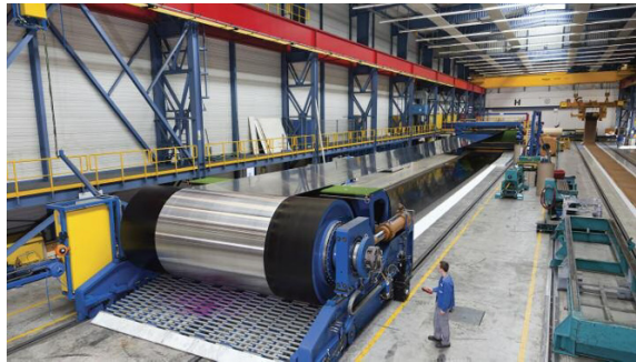
Fig. 13.19 Endless steel belt, moving between two rotating drums
