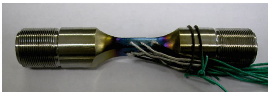
Fig. 3 Dummy specimen instrumented with multiple thermocouples at different locations to determine axial and circumferential temperature gradients
