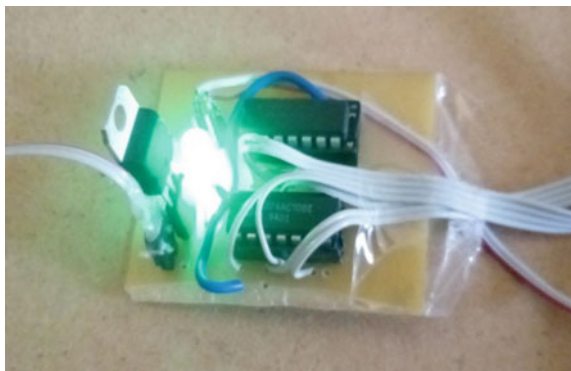
Fig. 8 Logic converter to H-Bridge motor driver (if the logic inputs to H-Bridge is logic '11' then the link is short circuited to avoid this we used the above shown converter which passes logic '00' when it gets logic '11' combination)
