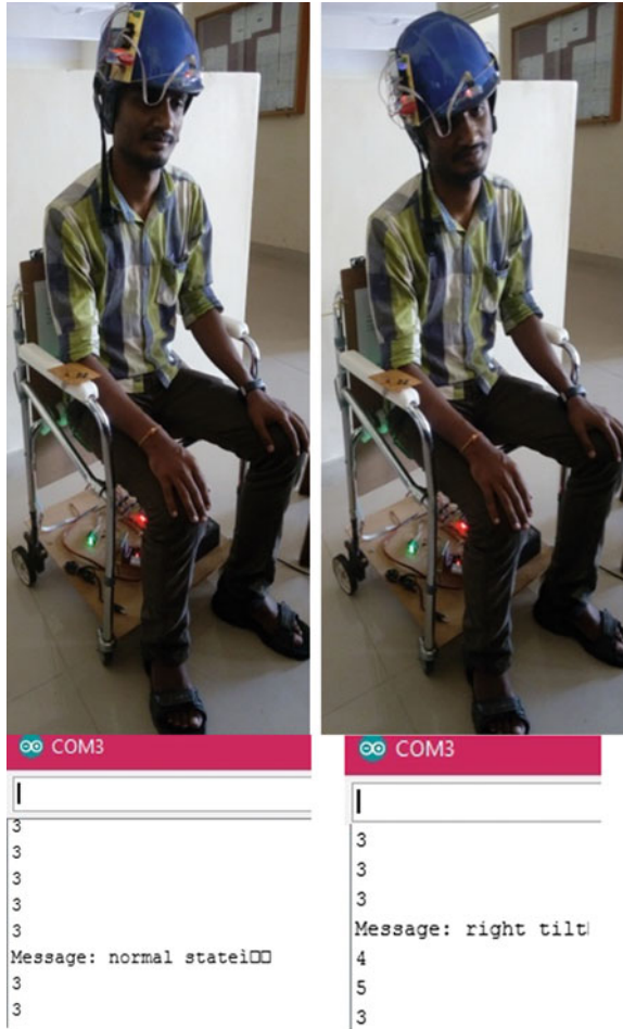
Fig. 14 Module testing for RIGHT tilts
