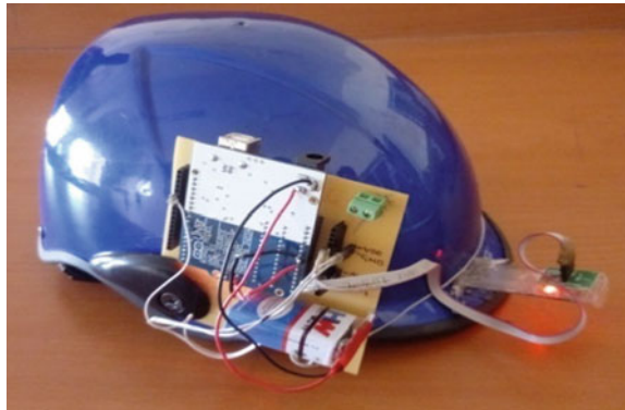
Fig. 4 Implementation of head control unit
