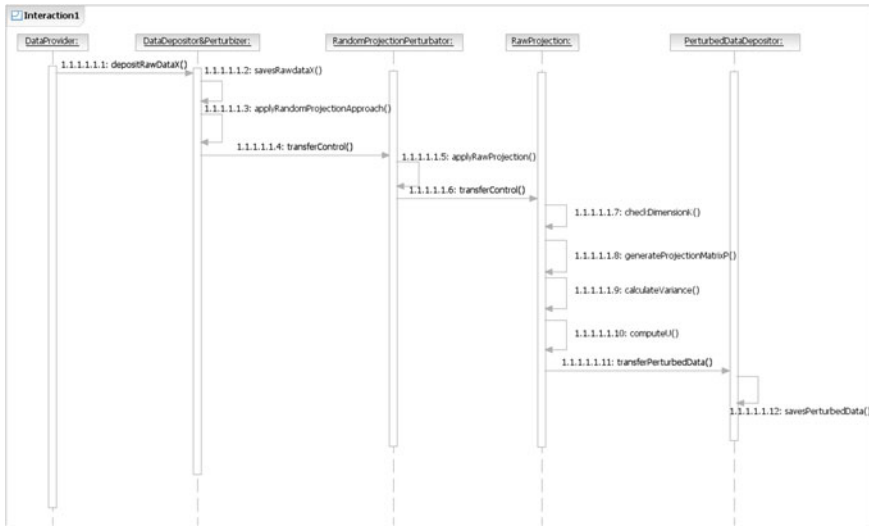
Fig. 10 Sequence diagram of Row-wise Projection Perturbation
