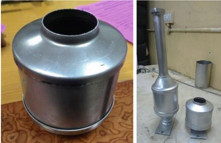
Fig. 5 Converters outer shell
