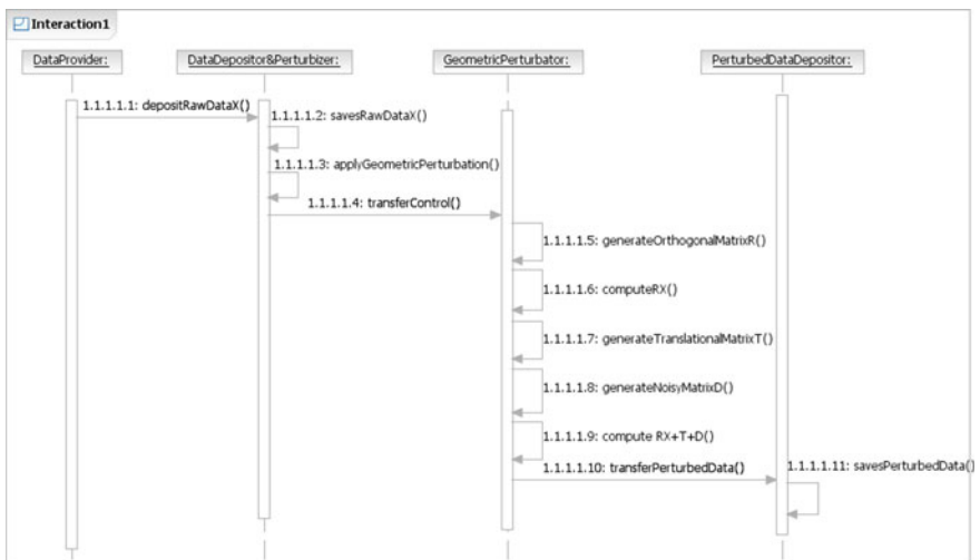
Fig. 9 Sequence diagram of Geometric Perturbation approach
