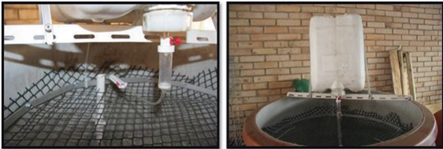
Fig. 3.16 The infusion applicator for bio-reagents used in the cartridge construction for containers of V = 20 L
