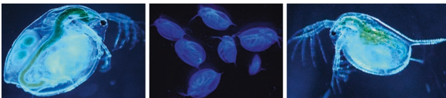
Fig. 18.10 Daphnia sp. during acute toxicity bioassay (type: Fluo-tox)
