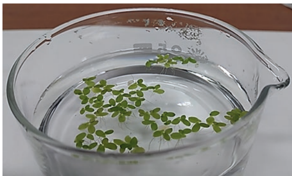
Fig. 18.5 Lemna minor toxicity bioassay (classical methods)
