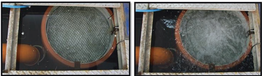
Fig. 3.15 Small-bubble aeration—formation of water–air mixture (bioreactor with the bed during the hydraulic tests). Phases with aeration and without aeration
