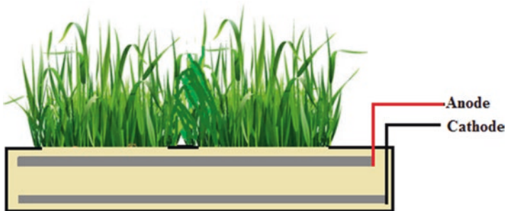
Fig. 17.6 Rooftop plant MFC
