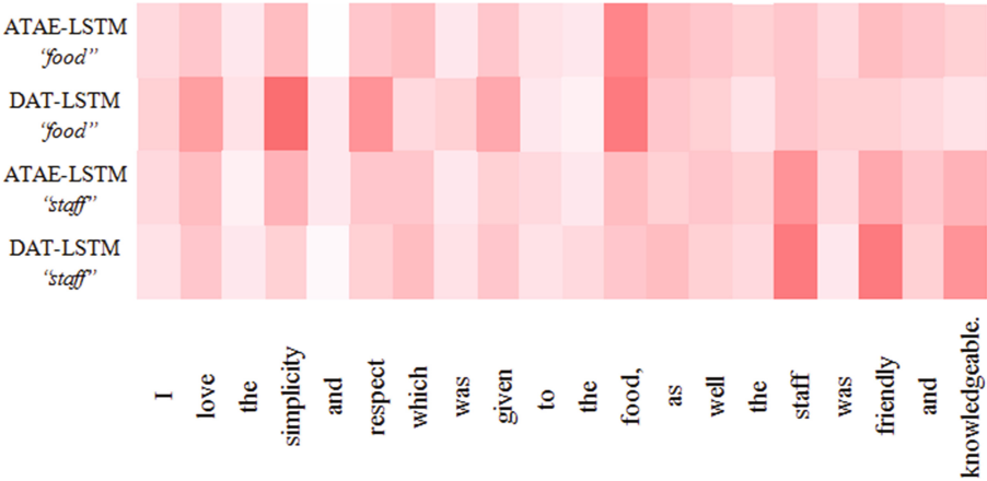
Fig. 4. Changes of attention weights in different models of the mentioned targets, “ food ” and “ staff ”.
