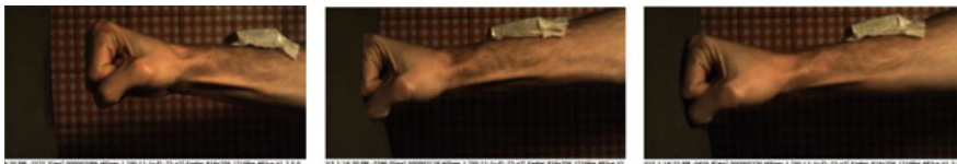
Fig. 1 Wrist-mounted sensor before impact (left); the sensor at time of impact (middle); the sensor orientation changes immediately following impact (right)
