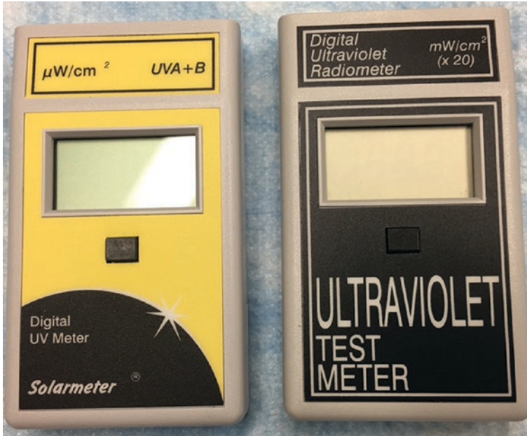
Fig. 14.2 Ultraviolet meters. Small, handheld, portable, battery-operated meters can be used to measure the amount of damaging UV radiation present outdoors or indoors enabling the patient to know when and where to protect themselves
