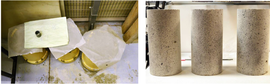
Fig. 3. Cylindrical specimens during the curing (at the left) and after the paint spraying for DIC (at the right).
