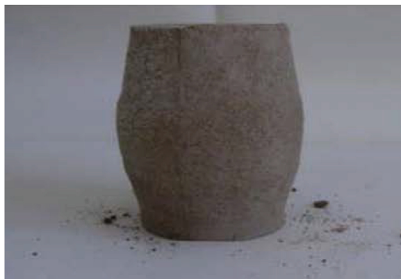
(b) Failure form of WIRFC
