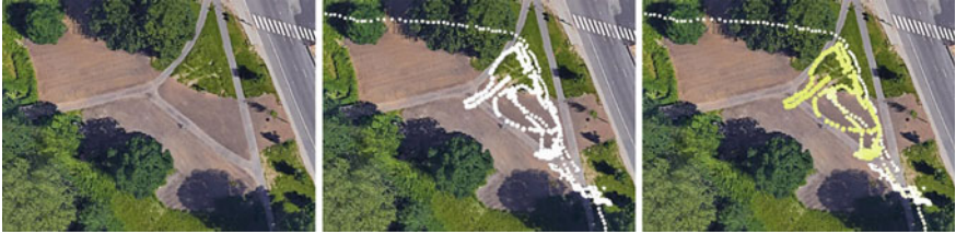
Fig. 7. From left to right : the site; sampled points mapped to the environment; a simple visualization of gas sensor data
