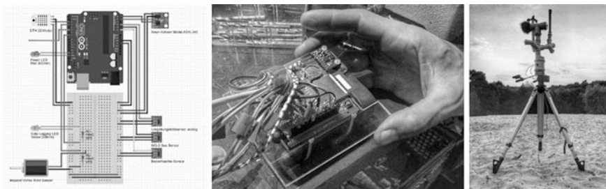
Fig. 1. Images and diagrams of the prototype Arduino-based mobile data logger for the field station project
