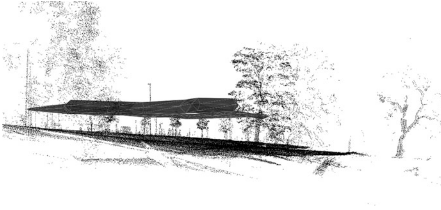
Fig. 10. Perspective view of volumetric representation of sound levels on site
