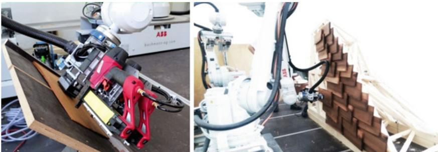
**Fig. 8.** *Left* Robotic scanning and gripping. *Right* Mounting and fixation of timber panel. We used hand-split timber panels of variable widths between 8 and 30 cm and a fixed height of 60 cm
